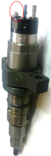
Broken magnet pin
