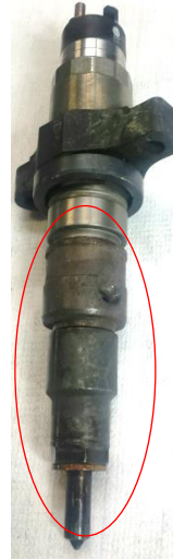
Heavy corrosion on the outside
